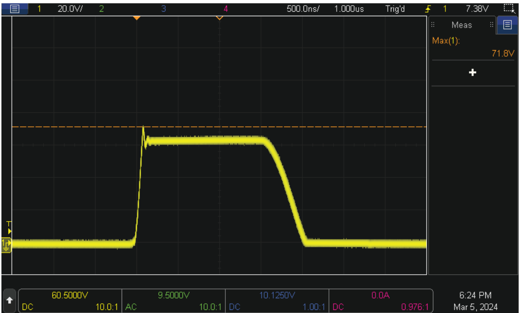
Figure 20. Voltage of Secondary Forward Diode (D7) at Full Load
