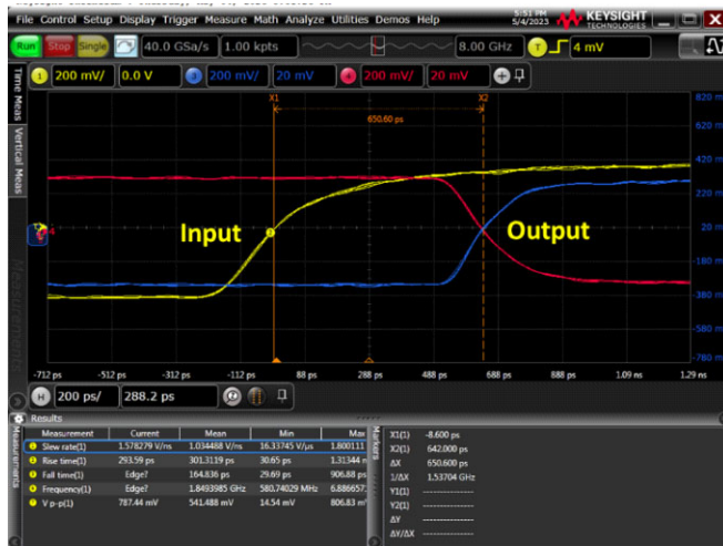
Figure 10. Sample Propagation Delay for LVPECL Output
