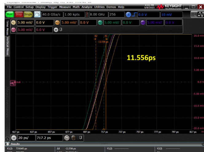
Figure 13. Sample Output-to-Output Skew for LVDS Output
