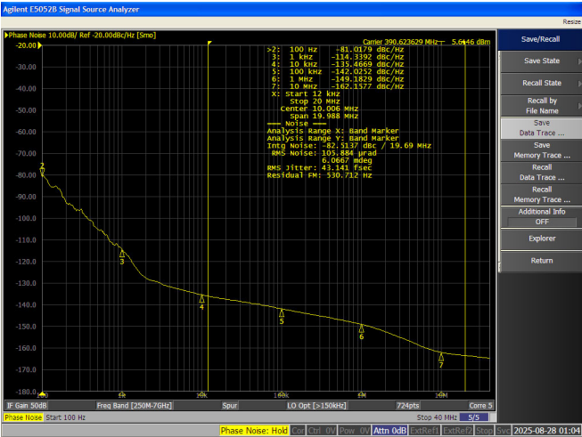
Figure 10. 43 fs RMS Jitter for 390.625 MHz SerDes Clocks
