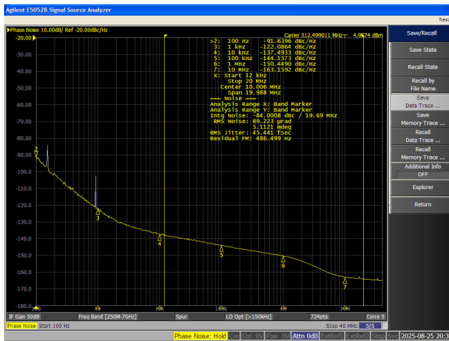
Figure 11. 45 fs RMS Jitter for 312.5 MHz SerDes Clocks
